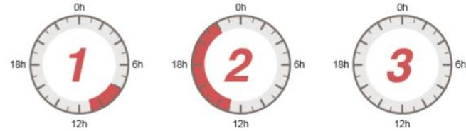
With 3 definable time periods, users can freely set the battery discharge time within the range of 00:00 to 23:59. During the time set by the user, the inverter will give priority to the battery inverter to carry the load, and if the battery power is insufficient, the inverter will automatically switch to mains power to ensure stable operation of the load.
