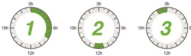
With 3 definable periods, the user can freely set the mains charging/supplying power time within the range of 00:00 to 23:59. During the time period set by the user, if PV energy is available, PV energy will be used first, and if PV energy is not available or insufficient, utility energy will be used as a supplement.
